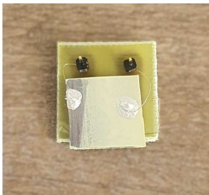
Figure 5. Photograph of the fabricated multilayer PZT-based touch sensor.
